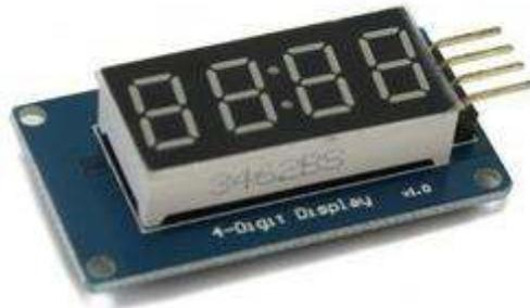
TM1637 is a chip for driving 7-segment displays. There are several modules using this chip to form a 4 digit numerical display module. TM1637 has also keyboard input capability, but is not used in this module.
