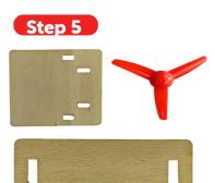
Now, snap board 6 onto board 4, snap board 7 onto boards 4 and 3, and slide the red fan blade onto the motor's spinning stick.
