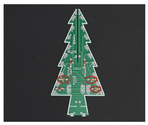
Step 2: Install 3pcs 10K Metal Film Resistor on R1,R3,R5
