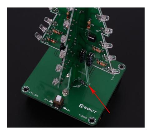
Step 18:Install the top LED.Note the positive and negative of LED.At this
