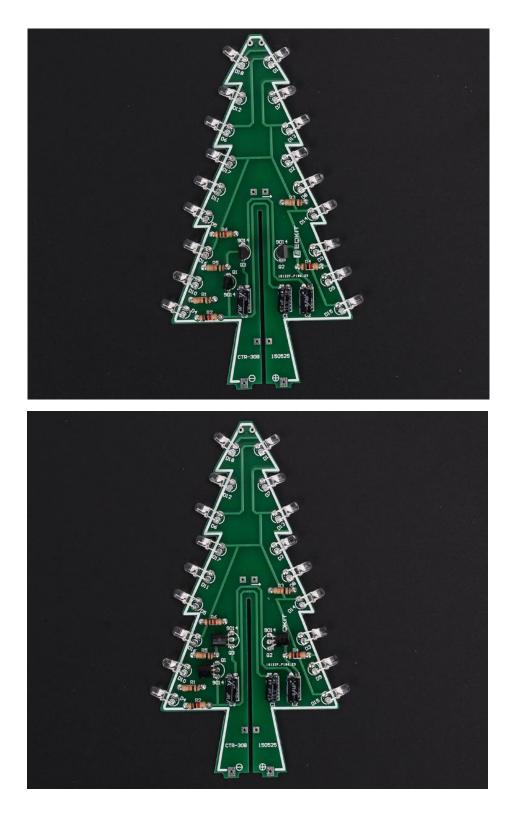
Step 11: Install 3pcs TO-92 S9014 Transistor
