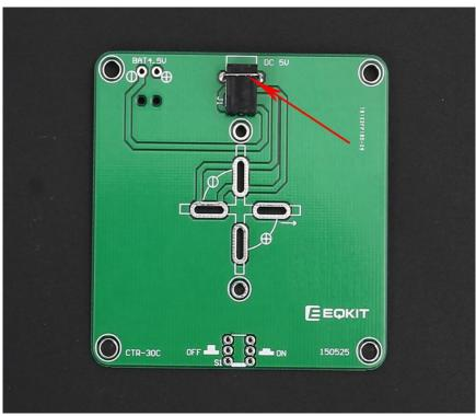
Step 15: Install 1pcs Self-Locking Switch. Note the direction of switch.
