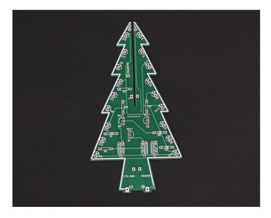
Step 1: Install 3pcs 1K Metal Film Resistor on R2,R4,R6
