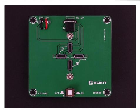
Step 17: Fixed CTR-30A and CTR-30B on CTR-30C.Align the two positioning heads and then fixed with tin.
