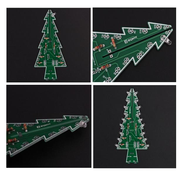
Step 5: Install 3pcs 47uF 16V Electrolytic Capacitor
