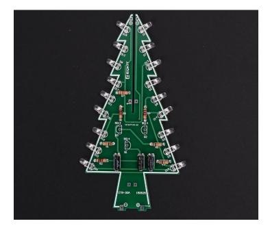
Step 6: Install 3pcs TO-92 S9014 Transistor
