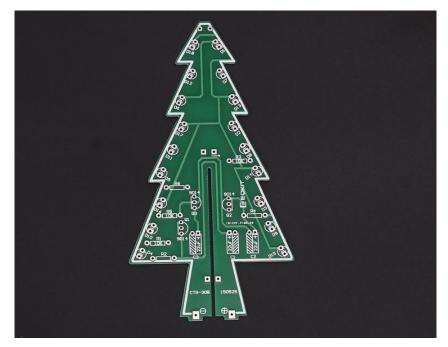
Step 7: Install 3pcs 1K Metal Film Resistor on R2,R4,R6
