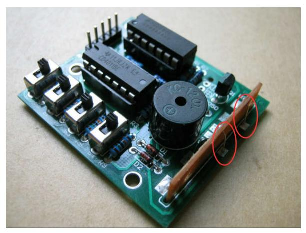
Step 6: Install 4 toggle switches and buzzer
