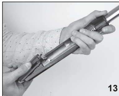
13. Pull back and remove the mechanism
