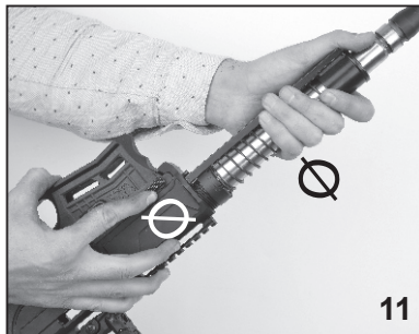
11. Turn the bolt catch lever.
