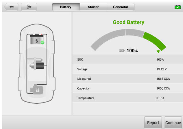
Figure 11-6 Battery Test Results Screen
