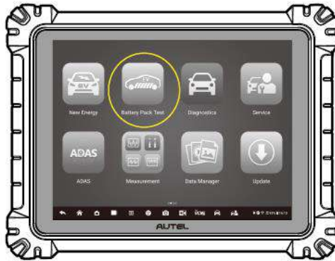
Figure 5-5 Tap Battery Pack Test
