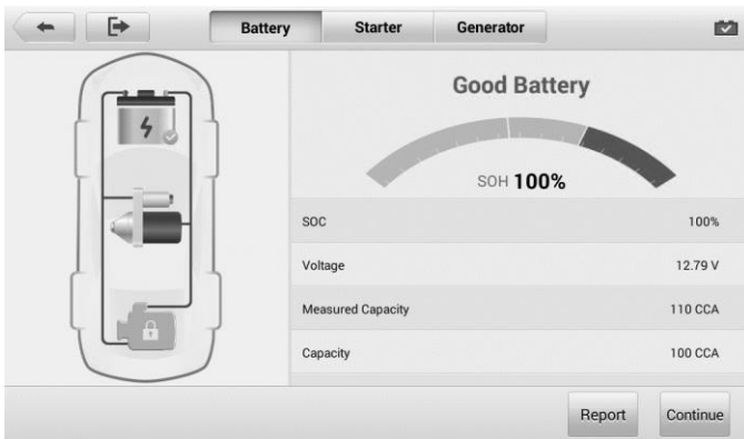
Figure 7-7 Sample Battery Test Results Screen
