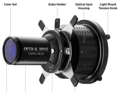
Gel Ring Clip Focusing Lens Lens Release Tab Light Cutting Leaves (4)
