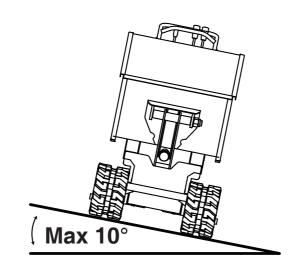
In figure the maximum values for the latitudinal and longitudinal slopes of the terrain are shown on which it is possible to work. These conditions must never be surpassed to avoid the risk of overturning.
