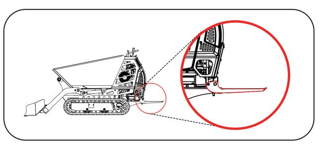
During the driving of the machine and during the work, is necessary utilize the footrest platform in open position to prevent risks.
