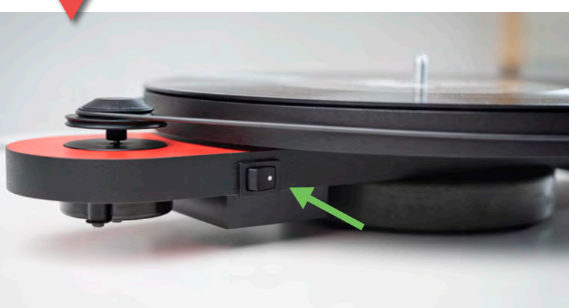
16 Turn the motor on.
