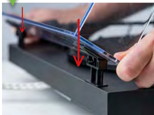
5 Slide the dustcover into the turntable.
