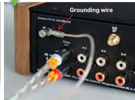
7 Connect the RCA cable to your amp.
