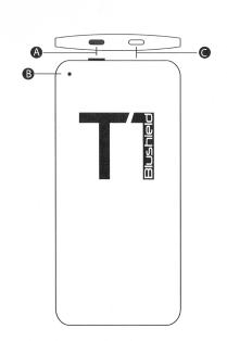
ON/OFF button Red/Green LED indicating function/charge USB C charging port The T1 carries a limited warranty for a period of 1 year. This does not cover misuse, modification or neglect (dropping, water damage). If a claim is to be made all postage costs are to be covered by the customer. A Blushield distributor will decide whether to repair or replace product depending upon the fault.
