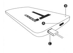
Once the USB charging head is inserted **(a)** the LED **(3)** will flash red indicating that the T1 is charging.
