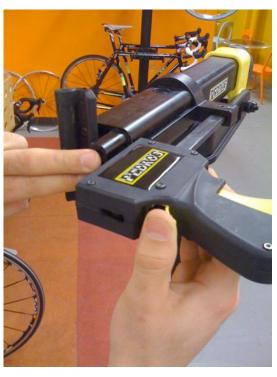
Step 4: Slide on the new clamp handle assembly over both the clamp slide and clamping shaft. Make sure the clamp lock lever is in the open position before installing. Refer to step 3 photos for correct orientation.
