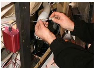
**STEP 2** - Unscrew nut and then unplug on/off connection from amplifier
