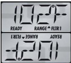
Allows the user to flip the display with a single button press.
