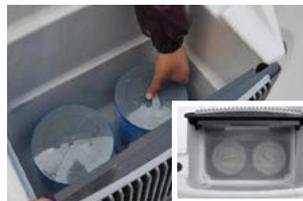
**Step 4.** Unscrew the two filters and replace with the new filters and rescrew into position.
