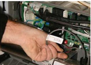
**STEP 5** - Unplug sensors plug from circuit board - Pinch tab down before pulling out plug.
