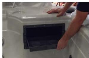
**Step 2.** Remove the filter tray in order to access the filter compartment.
