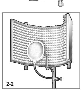
**4.** Securely clamp tight **Pop Filter (B)** on the **Speaker Stand (E)** just below the **Microphone Isolation Shield (A)**. See **2-2**.
