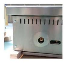
Unscrew bolts and pilot valve, then remove the manifold.
