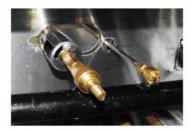
Replace the orifice fittings into the valve.
