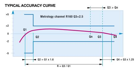
The dynamic range is defined as the Ratio (R) between the nominal and the minimum flowrate. The MID approval proves the Aquadis+ HW real capacity to withstands to higher nominal flows (Q3 > Qn).
