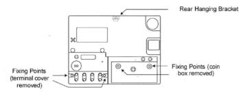
When installing the meter, initially it should be hung from the rear hanging bracket using a suitable round headed screw. The screw depth should be adjusted so the head fits snugly under the hanging point and the meter is help firm against the wall. Once hung, ensure the meter is level then mark and screw the meter to the wall securely using the four fixing points; two are located under the grey terminal cover and two are under the coin box (see drawing above).
