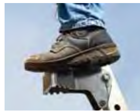
Steps are used to access the head to untangle ropes or attach additional gear without having to lower the system.
