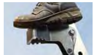
Steps are used to access the head to untangle ropes or attach additional
