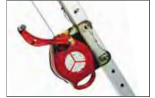
Type 3 Fall Arrest Block. Inertia reel with wind up/down mechanism. 8mm galvanised steel cable with twist lock, fall-indicating, swivel karabiner. 15 m, 1 person fall arrest.
