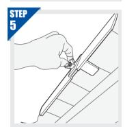
**ENSURE WING NUT IS TIGHTENED TO SECURE BOTTOM** TAB AS SHOWN
