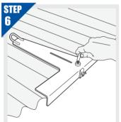
**ENSURE L BOLT IS TIGHTENED** ONTO ROOFING IRON TO CLAMP ANCHOR TO ROOFING IRON.
