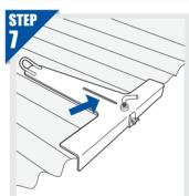
**SCREW IN A ROOF SCREW** THROUGH THE SLOTTED SECTION IN FRONT OF THE L-BOLT AS HIGHLIGHTED BY THE **BLUE ARROW**
