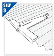
SIT THE ANCHOR ON TOP **CORRUGATION OF ROOFING IRON AS SHOWN**
