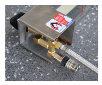
**4.** Place new burner (1) into rear burner slot of Snappy King, followed by the existing burner (2) in the front burner slot.
