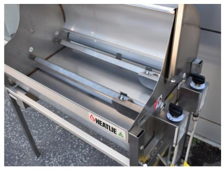
**5.** Attach the two burners together via quick connect fitting (3). Pull the silver gripped part back while inserting the fitting. Release this, then twist the black gripped ring to lock in place.
