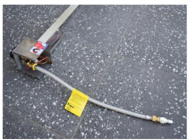
3. Attach hose and regulator (4) to the new burner (1).
