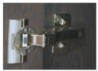
Start by removing the Zuster tag off the hinge plate to reveal the phillips head screws.
