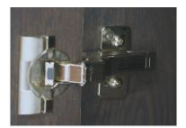
Start by removing the Zuster tag off the hinge plate to reveal the phillips head screws.
