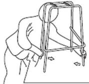
IF THE LEG IS UNEVEN AFTER ASSEMBLY, PLEASE LOOSEN THE SCREW, ADJUST THE ANGLE, AND THEN TIGHTEN IT.
