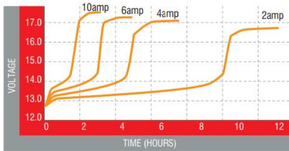
Charge characteristics from 20% DOD, 31DC-205
