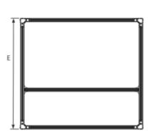
A: Boom lengths: 3 or 4 m B: Height 2.33 m (2.36–2.46 m adjustable foot is mounted,
