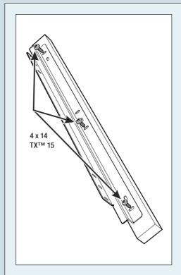
Mount the panel onto the angle bracket using three 4 x 14 screws.
