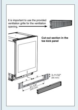
The cut-out section in the toe kick panel must be centered in relation to the appliance and in the uppermost part of the toe kick.
