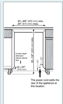
Height when adjustable feet have been screwed Free length of the power cord in as far as they will go.
