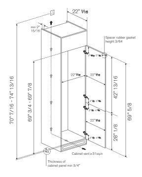
The refrigerator is installed on the cabinet base shelf and not on the kitchen floor.
