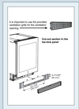
The cut-out section in the toe kick panel must be centered in relation to the appliance and in the uppermost part of the toe kick.
