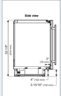
23 - 5/8" (600 mm) min. 24" (610 mm) max. The power cord exits the rear of the appliance at this location.
