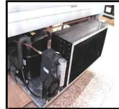
PULL OUT CONDENSING UNIT ON SELF CONTAINED
