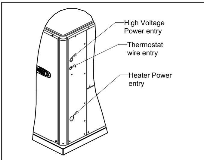
**Figure 2. Typical Field Wiring**
