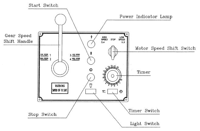
NOTE: TO START THE MOTOR, PUSH START BUTTON, THE SPEED SELECTOR HANDLE MUST BE AT THE NUMBERS, INDICATING A SPEED, NOT AT AN INTERMEDIATE POSITION.
