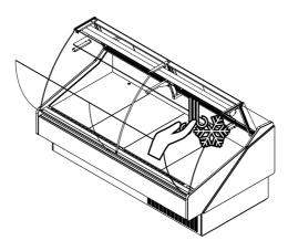
6 - Check air movement in the anti condensation system.
