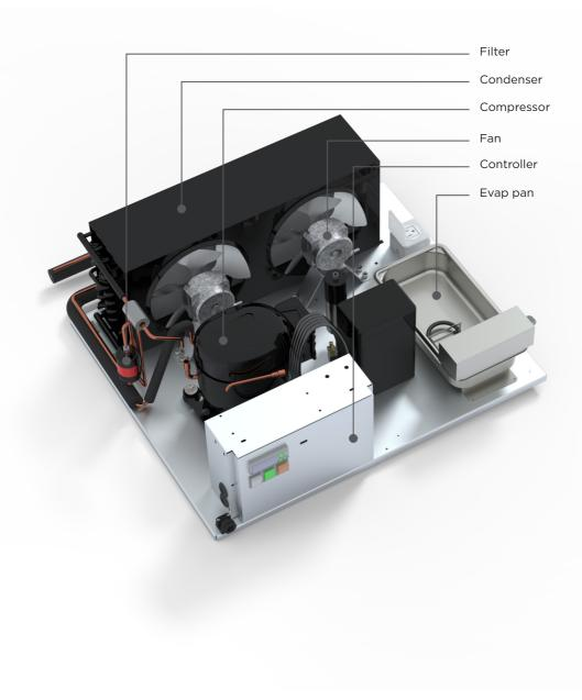
All self contained KFM series use the following equipment: capillary tube, finned coil ventilated systems (condenser/evaporator), hermetic compressor, electrical water evaporation system.
