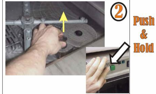
1] Open the door. 2] Remove the Over-flow tube, 3] Drain unit. Push and hold white button.
