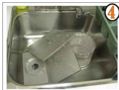
Clean the screens and wash tank of debris. Rinse wash tank. Be careful not to push food debris down the drain.
