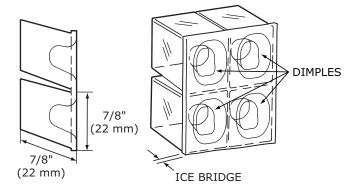
Your clear ice machine is pre-set to produce ice between the optimal dimensions illustrated below:
