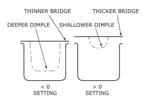
Ice thickness adjustments are made using the control panel as follows:
