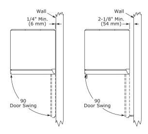
Units have a zero clearance for the door to open 90°, when installed adjacent to cabinets.
