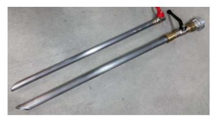
The steam outlet lance is drilled into the end of the liner and must be pushed in to the sole (liner bottom).
