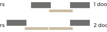
Track length: Twice the door opening width Fixing: Soffit or Wall Mount
