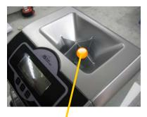
Motorized intermittent rotating disk at bottom of hopper feeds coins into internal sorting vessel in controlled batches and ribs separate coins into quadrants to help control flow.
