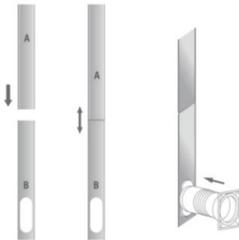
**STEP 4:** Open the window and place the window kit on the inside edge of the window. Adjust the window seal plate to the width of the window. Once secure, close the window to secure it in place.
