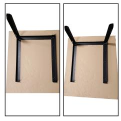
On one side from step 2, attach the Face Rails (C) in the opposite corners from the (B) rails.
