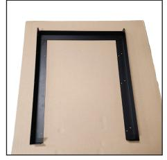
Lay out 2 Legs (A) and attach 1 side rail (B) to the corners of each leg (A). Do this to create 2 sides of the stand.
