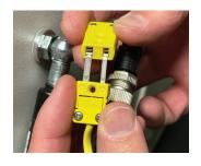
STEP 5 Then connect the yellow plug. Both plugs are directional and will only fit together one way. Do no attempt to force plugs together.
