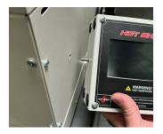
STEP 2 Insert the threaded rod into the threaded hole on the right side of the kiln.
