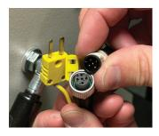
STEP 4 Next, take the cord connected to the control box and connect the black and silver plug. Make sure to align the locating marks on the plug before tightening the connector.
