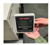
STEP 3 Use the knob attached to the control box to tighten the control box until it is snug.
