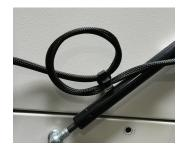
STEP 6 Now secure the control box wire with the wire retainer on the side of the kiln.
