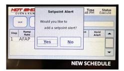
Adding a setpoint alert will sound an alarm when the setpoint temperature is reached.
