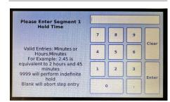
Enter segment hold time (Soak) in minutes or hours. Input examples below: 5 = 5 min, 5.0 = 5 hrs, 5.45 = 5 hrs and 45 min, 90 = 1.5 hrs
