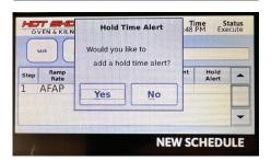
Adding a hold time alert will sound an alarm when the segment hold time has completed.
