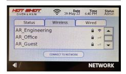
On the network screen, press "Wireless" and a list of available networks should appear. Select the appropriate network and press "CONNECT TO NETWORK"
