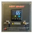
Press the "P" button and using the up/down arrows, set the desired temperature. When the Heat Enable switch is turned on the oven will ramp to the setpoint and hold until the oven is shut off.
