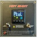
Press the "P" button one time until "Ptol" appears (This stands for tolerance). This setting controls how closely the internal temp follows the program.
