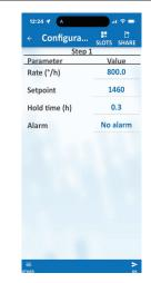
Begin to enter in your parameters. First, enter your RAMP RATE (DPH). Then, enter in your desired SET POINT TEMPERATURE. Finally, enter in your desired HOLD TIME. If you choose to have an ALARM, click on the alarm section and choose when you would like the alarm to go off. To enter in STEP 2, click on "OK" on the bottom right corner.
