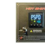
Press the "P" button one time so "PSP0" appears. This will be the first temperature setpoint of the program.
