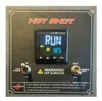
Press the "P" button one time to get to the "RUN" screen. Make sure it is set to "YES."
