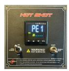
Press the "P" button one time until "PE1" appears (This stands for alarm). If an alarm is desired in this segment, set to "1."
