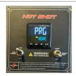
Using the up/down arrows, toggle to "NONE."
