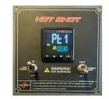
Press the "P" button one time so "Pt1" appears. This will be the desired time between the 1st and 2nd setpoint of the program. 30 minutes is shown above.
