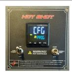
Press and hold the "P" button approx. 8 seconds until the "CFG PROG" screen appears.
