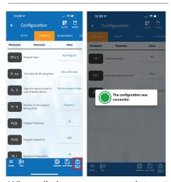
When all changes are complete, tap "Send to Device." "The configuration was successful" will appear when the data transfer is complete.
