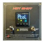
Press the "P" button one time until "Ptol" appears. The setting controls how closely the internal temp follows the program.
