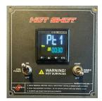
Press the "P" button until "Pt1" appears. This will be the desired time between the 1st and 2nd setpoint of the program. 30 minutes is shown above.
