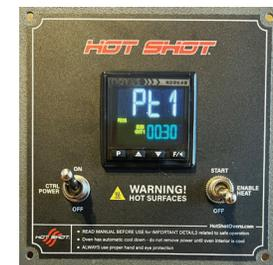
Press the “P” button until “Pt1” appears. This will be the desired time between the 1st and 2nd setpoint of the program. 30 minutes is shown above.
