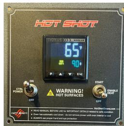
Using the up/down arrows, set the desired temperature. When the Heat Enable switch is turned on the oven will ramp to the setpoint and hold until the oven is shut off.
