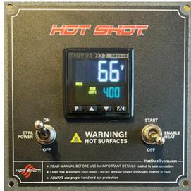
To run a simple temperature hold, start by turning the control power on.
