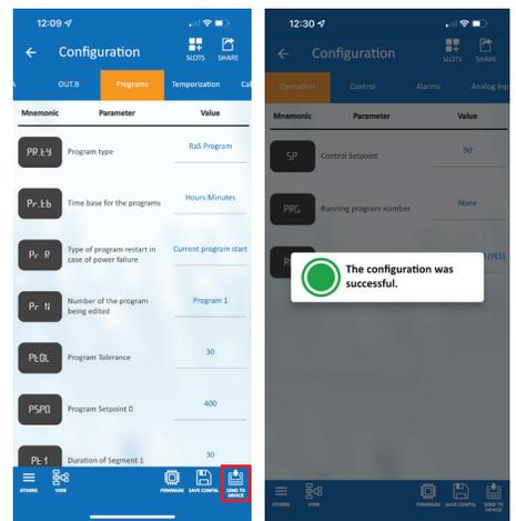
When all changes are complete, tap "Send to Device." "The configuration was successful" will appear when the data transfer is complete.
