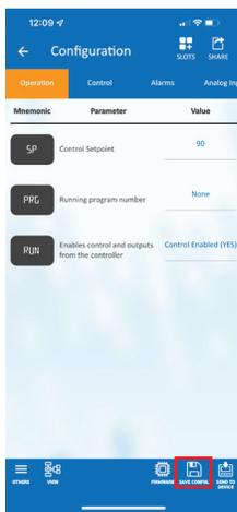
Save the current configuration in case you need to load the original programming back into the controller.
