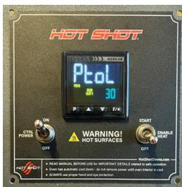
Press the “P” button one time until “Ptol” appears. The setting controls how closely the internal temp follows the program.
