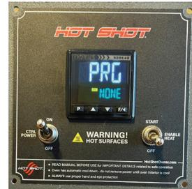
Using the up/down arrows, toggle to "NONE."
