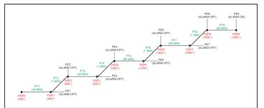
400°F for 30 minutes 800°F for 45 minutes 1200°F for 60 minutes 1600°F for 60 minutes 1800°F for 60 minutes
