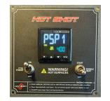
Press the "P" button one time until "PSP1" appears. This will be the second setpoint temp of the program. STEP 3:
