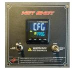
Press and hold the "P" button approx. 8 seconds until the "CFG PROG" screen appears.
