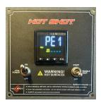
Press the "P" button one time until "PE1" appears. If an alarm is desired in this segment, set to "1."
