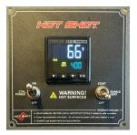
To run a simple temperature hold, start by turning the control power on. STEP 2:
