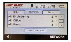
On the network screen, press "Wireless" and a list of available networks should appear. Select the appropriate network and press "CONNECT TO NETWORK" STEP 2:
